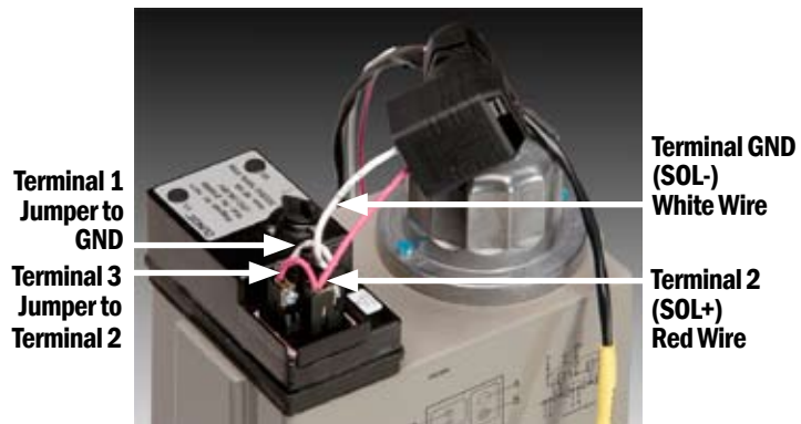
FUEL HARNESS TO ROP CONNECTIONS
